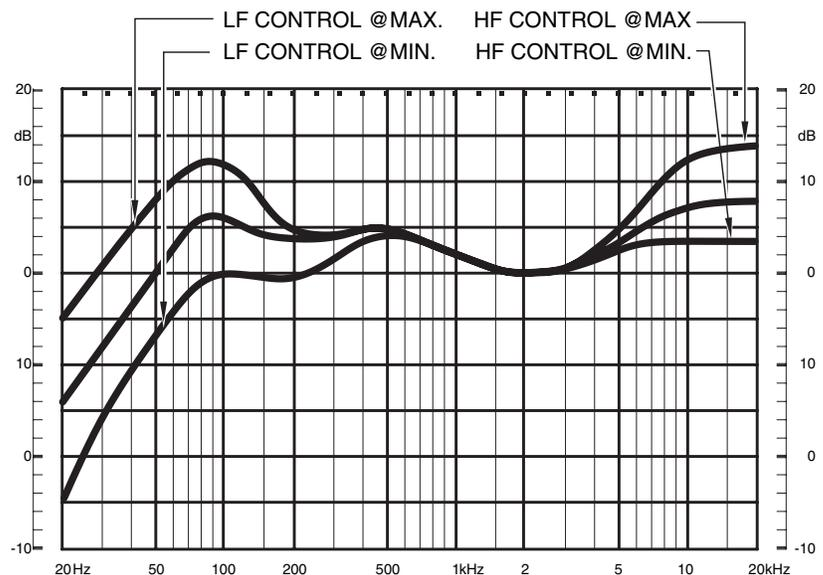
NOTE: CURVES SHOWN ARE WITH CAVITY CORRECTION SWITCH IN "WALL" POSITION AND THE SUB (LF CUTOFF) SWITCH 'ON'
